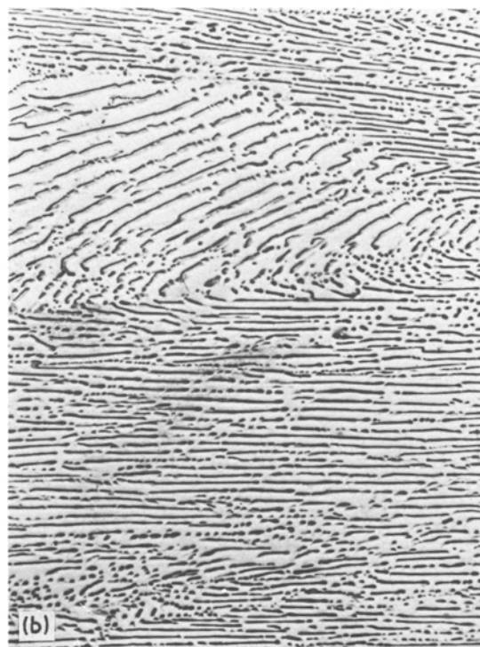
Figure 6 Eutectic structure (optical micrograph) on transverse (a) and longitudinal section (b) of Al–7.15 wt % Au specimen unidirectionally solidified at 2.55 \times 10^{-3} \text{ cm sec}^{-1} ( \times 200 ).
